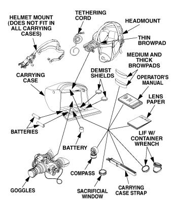
Figure 1-1. Night Vision Goggles (NVG), AN/PVS-7B and AN/PVS-7D (Sheet 1 of 3).
